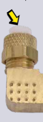
67219 1/4" Compression fitting for oil drippers with 1/8" NPT male thread (elbow)
