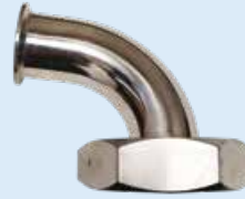
54824 3" bevel seat w/nut x 1½" tri 90 degree elbow, concentric
