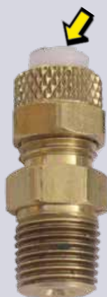
67218 1/4" Compression fitting for oil drippers with 1/8" NPT male thread (straight)
