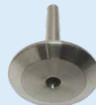
54865 2" x 4" probe well with ½" OD x .049 wall tubing
